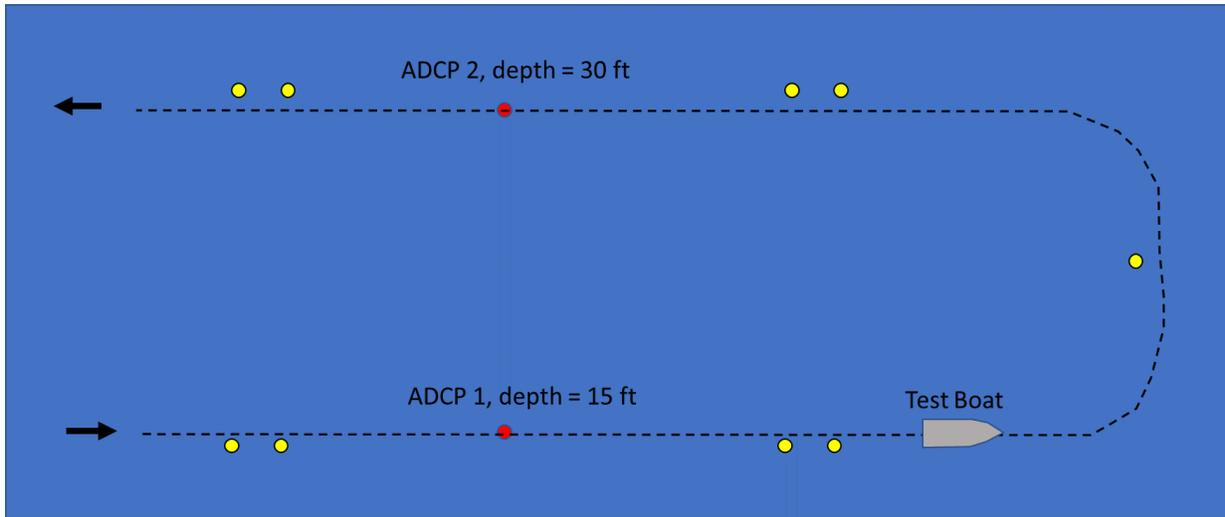
Figure 1. Schematic of the testing scheme. The test boat will travel a u-shaped track denoted by yellow buoys (circles) that passes over two bottom-mounted ADCPs deployed in approximately 15 ft and 30 ft of water.
