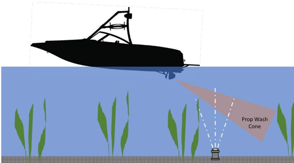
Figure 2. Conceptual drawing of propeller wash test with ADCP placed upward-looking.
